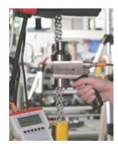
With the new CHTK tester for overload cutoff, NOSHOK offers a precise, durable and dependable tester for slip couplings on chain hoists. The CHTK provides a wide range of measurement, with high accuracy, low weight and ease of use.
