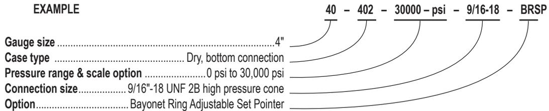
**9/16"-18 UNF 2B High Pressure Cone Connection**
