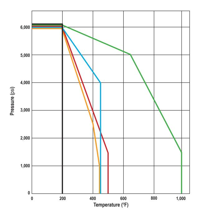
Steel needle valve with Graphite (P2) packing
