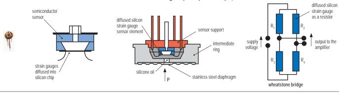
Sputtered Thin Film Strain Gauge Sensor (used in 100, 200, 612, 613, 615, 616, 621, 622, 623, 624, 625, 626, 627, 640, 650, 660, 800/810 Series - ranges 0 psi to 500 psi and higher)
